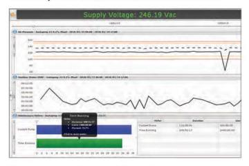
Plantnode can track any variable that changes over time, setting limits for an upper and lower condition. If a condition is exceeded, Plantnode can send a series of escalating alarms to the display board or alerts to key people.
